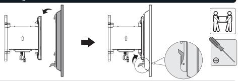
Lift and hook the TV onto the wall mount.
