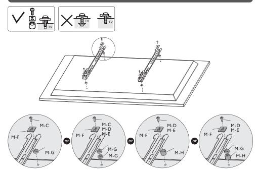
Note: Choose the appropriate screws, washers and spacers (if necessary) according to the type of screen.
