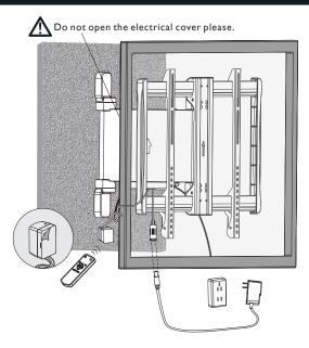
Do not plug into the power outlet until it is ready to be operated.
