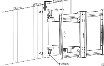
Align the big holes on the wall plate to the screws in the wall and lower the wall plate.
